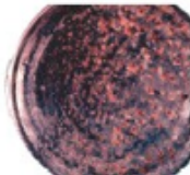
Sharp dents parallel to the rim
