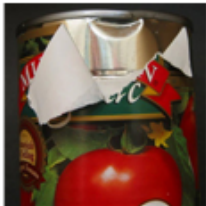
Sharp dents parallel to the rim
